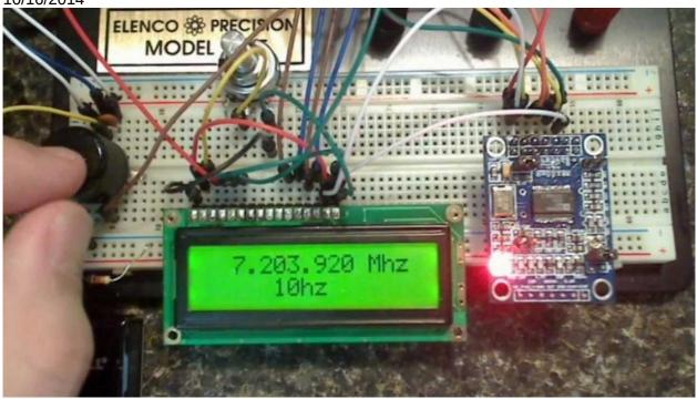
The heart of this circuit is the AD9850 chip. This gem is a 0-40 MHZ sine and square wave generator. What's used in the circuit above is a break out board version that is available on eBay for about \$4 - \$8 shipped.
